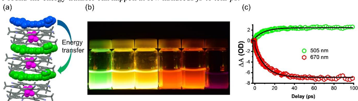
Figure 1: (a) small-molecule ionic isolation lattices (SMILES) structure, blue: energy donor, green: energy acceptor; (b) SMILES NPs with different emission color under 365 light illumination; (c) fs transient absorption decay traces monitored at energy acceptor in SMILES NPs.
