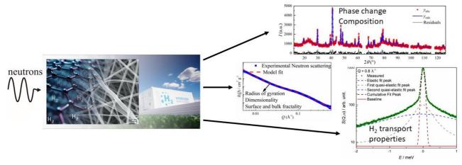
Scheme: A schematic of different neutron scattering methods yielding *in situ* information of different processes dealing with crystalline phase changes, adsorbent porous structure, and adsorbed phase transport properties.
