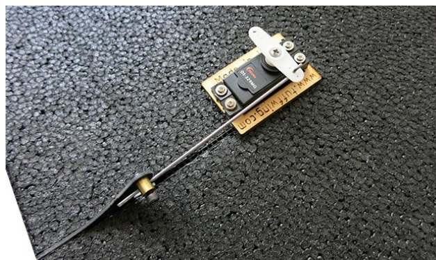
Image 3. Engine and rod used to move the support surface.
