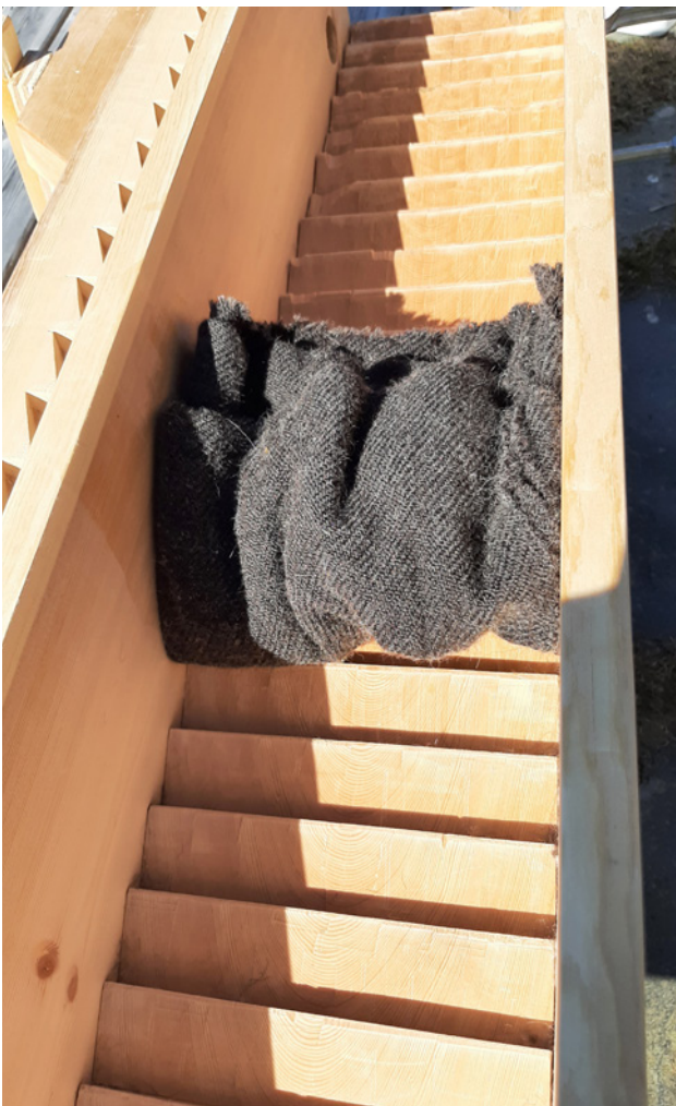
Photo 39. Folded fabric on the waulking board. Photo by E. Wendelbo
