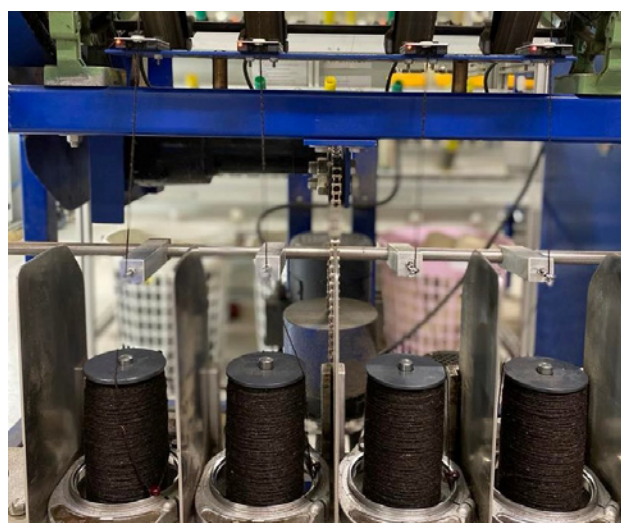
Photo 21. Plying process in the Selbu spinneri. Photo by M. Svorkmo Espelien
