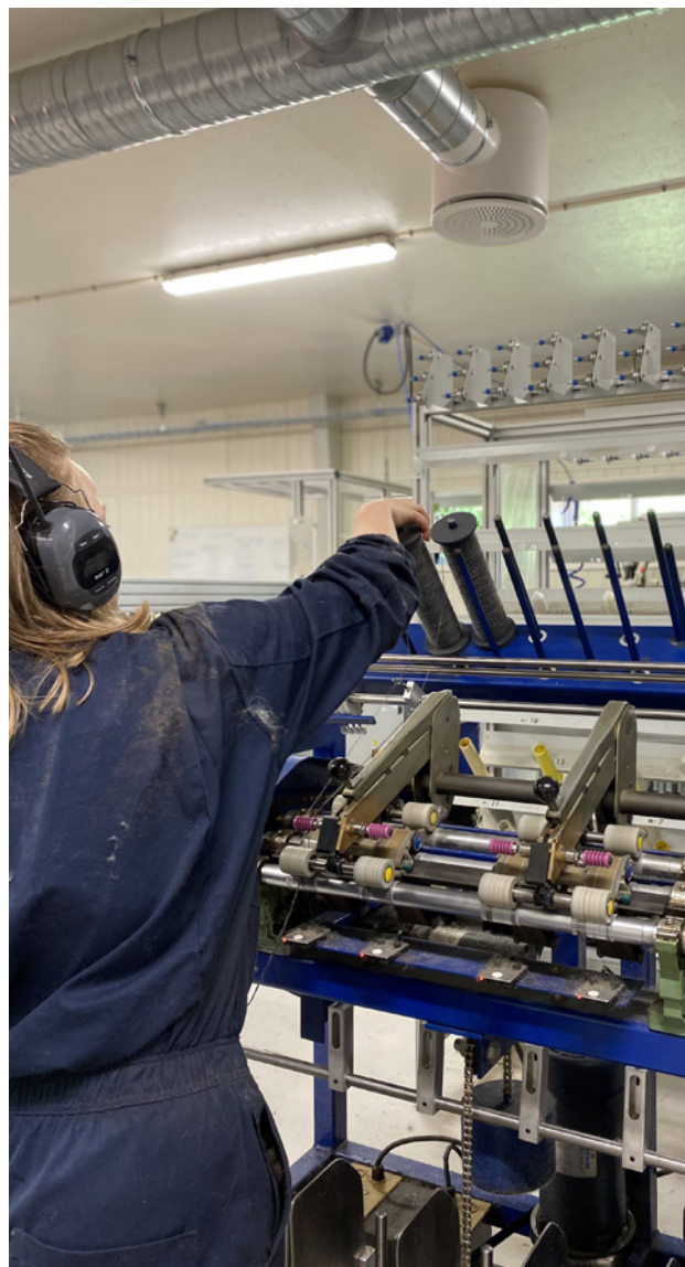
Photo 20. Plying frame in Selbu spinneri. Photo by M. Svorkmo Espelien
