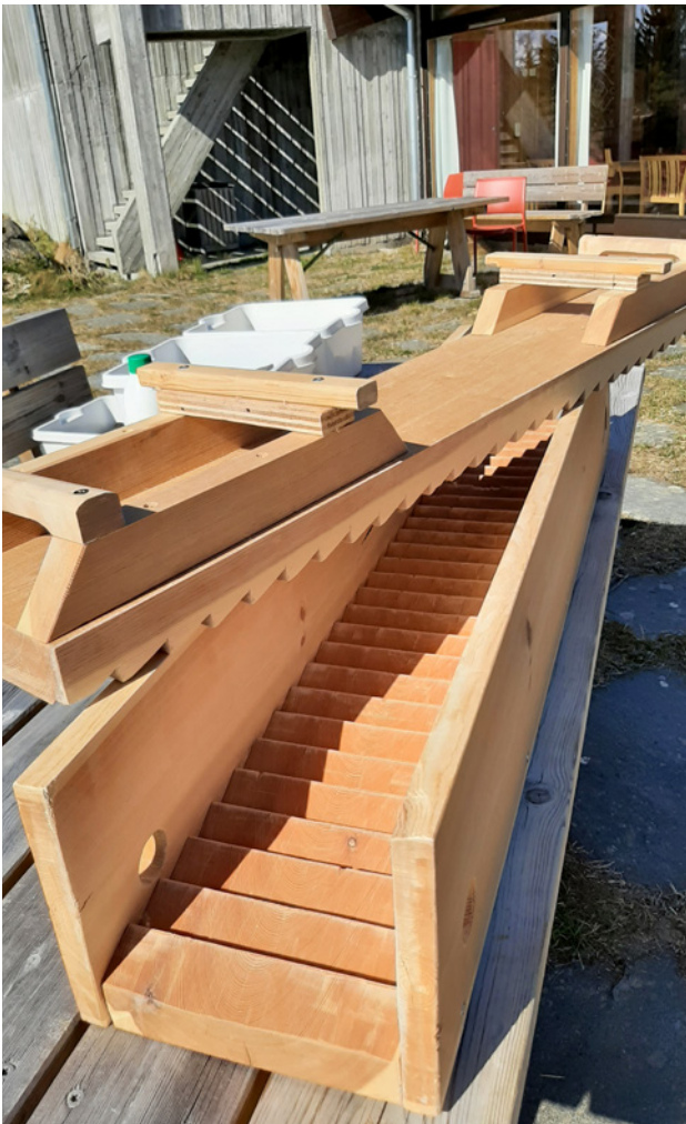
Photo 35. Homemade wooden box for waulking. Photo by E. Wendelbo
