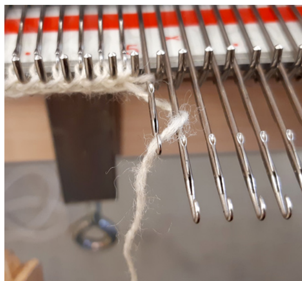
Photo 41. Creating loops on the knitting machine. Photo by L. Reinula
