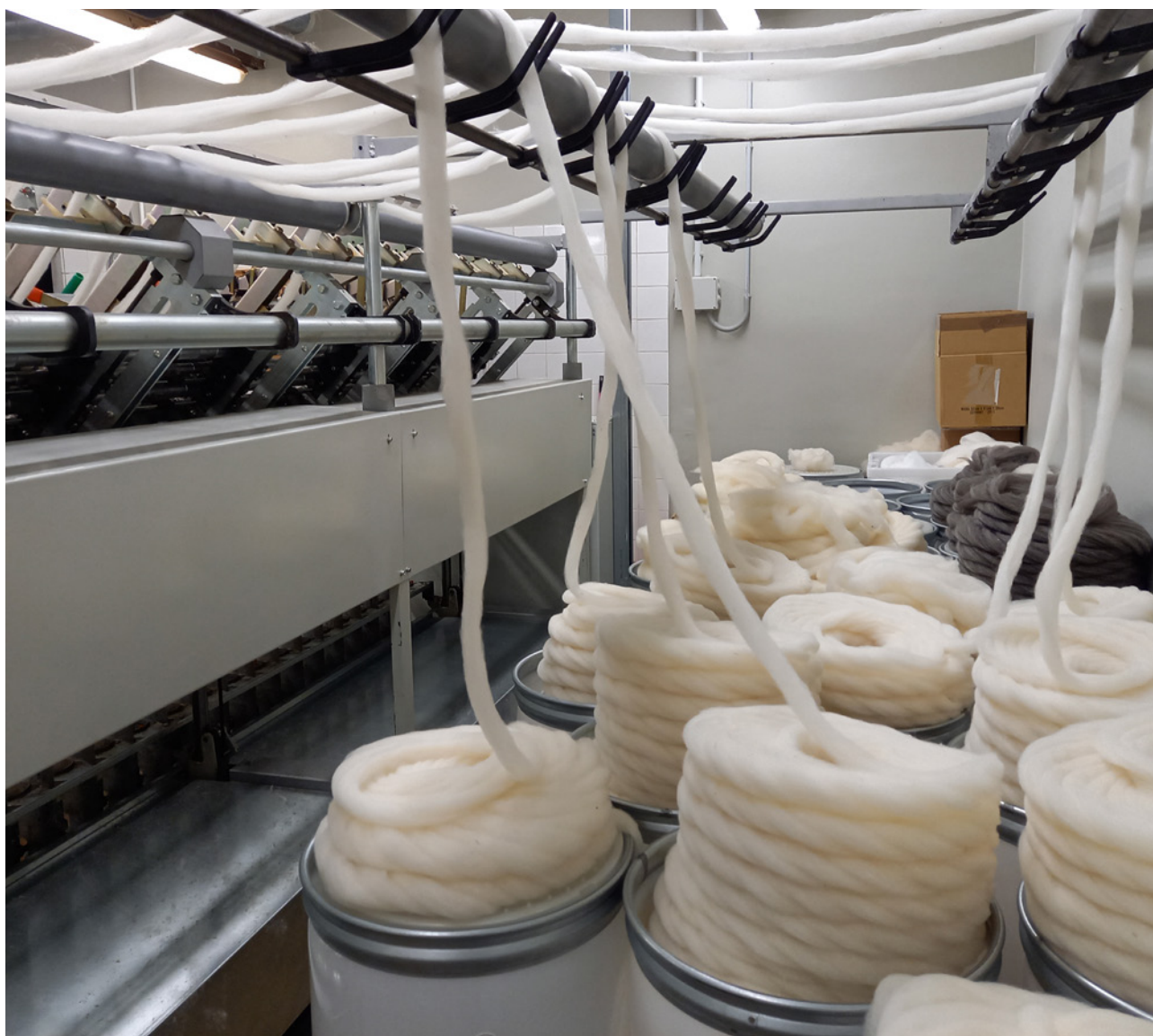
Photo 16. Slivers ready to spin in the back of the spinning frame in the Vilma wool mill. Photo by A. Kaljus
