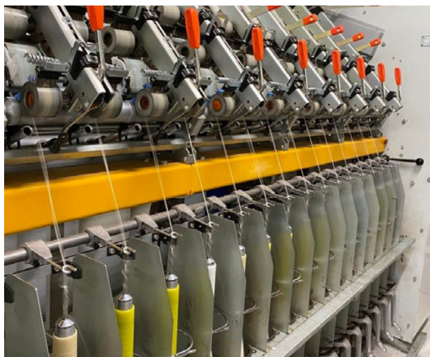
Photo 18. Spinning frame in Selbu spinneri. Photo by M. Espelien Blomli
