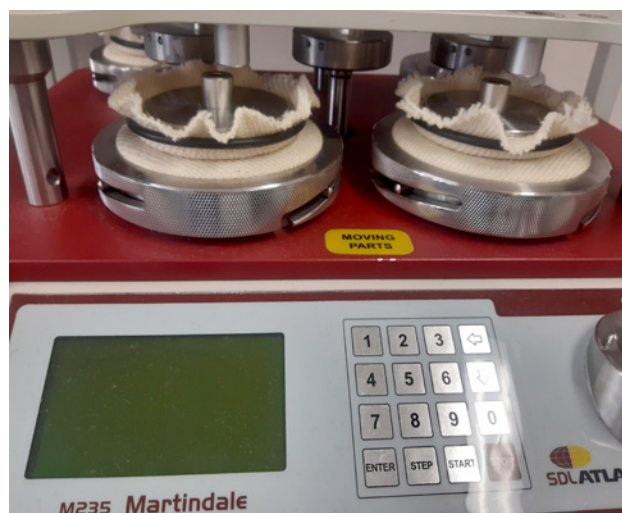
Photo 53. Pilling resistance testing. Photo by D. Tuulik
