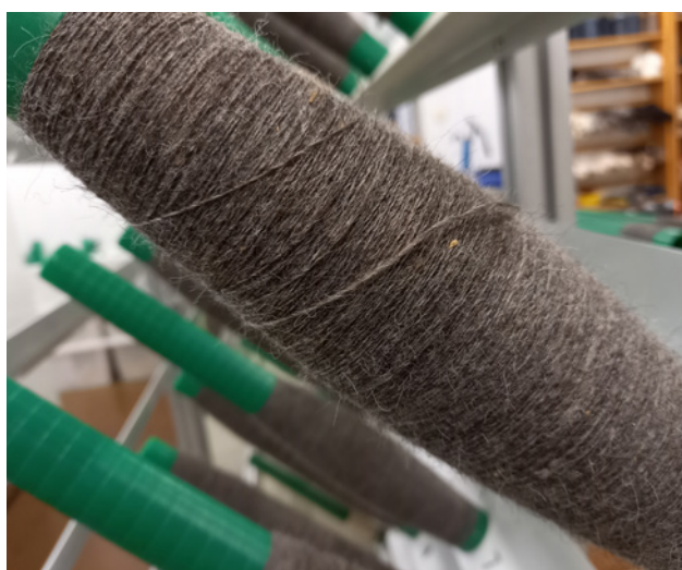
Photo 19. Single yarn waiting for plying in Vilma wool mill. Photo by A. Kaljus
