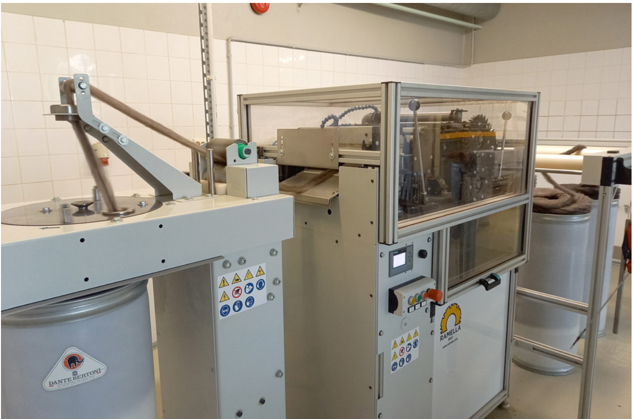
Photo 14. Pin-drafter in work in Vilma wool mill. Photo by A. Kaljus
