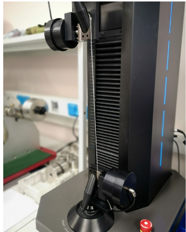
Photo 49. Measuring tensile strength of yarn. Photo by M. Beilmann
