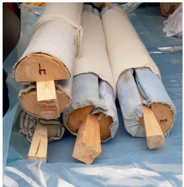
Photo 40. Final stretching of the fabric with the help of the wedges. Photo by E. Wendelbo
