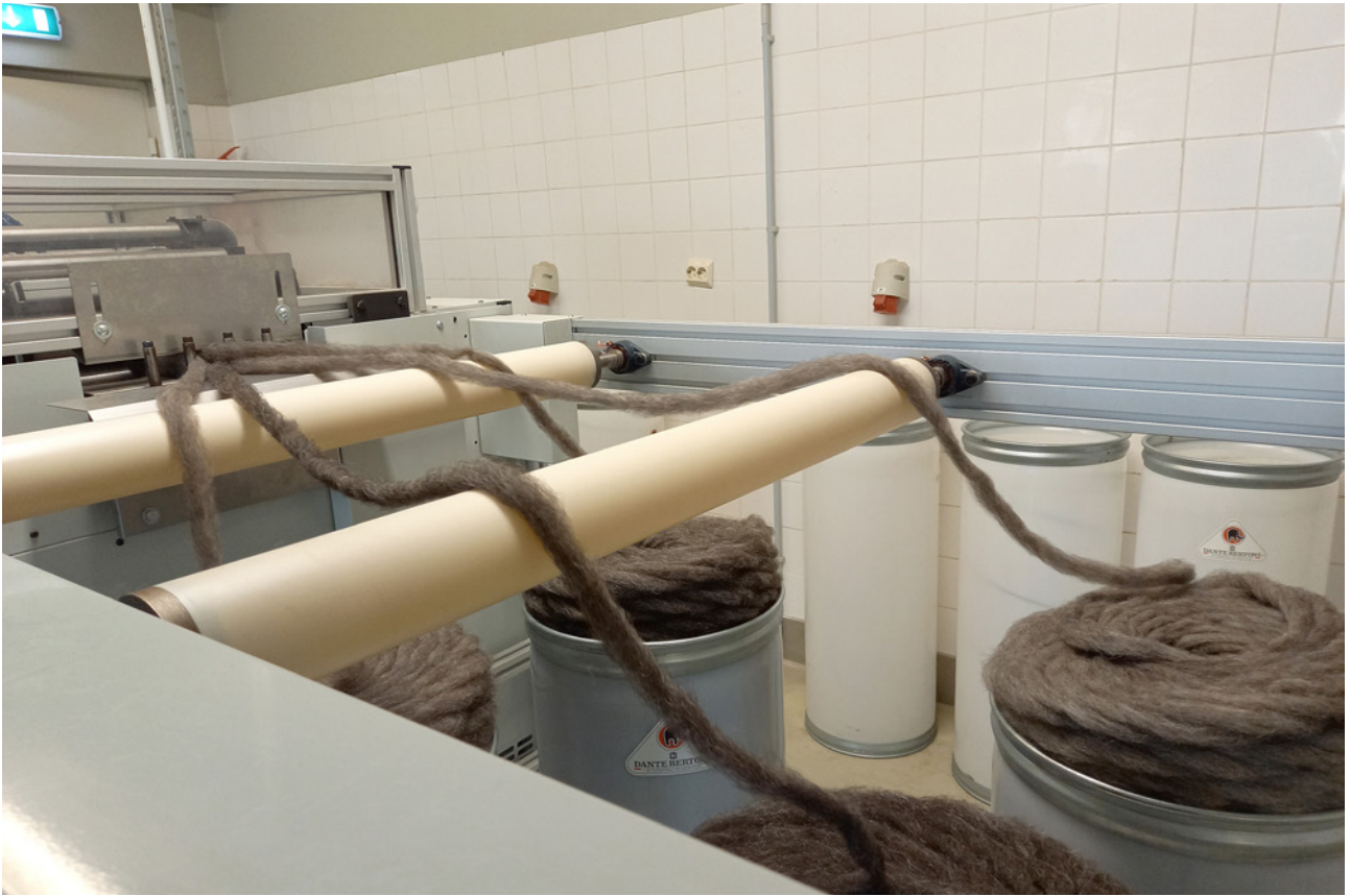
Photo 13. Pin-drafter in work in Vilma wool mill. Photo by A. Kaljus
