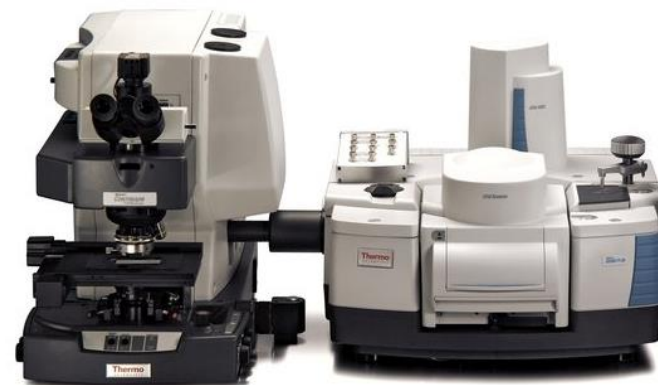
Thermo Fisher Nicolet™ Continuum™ Infrared Microscope (Photo: www.thermo.com/ ) (used with permission)
