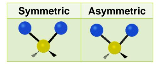
Bending (deformation) vibrations – bond angle changes
