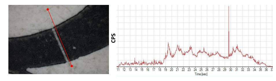
40 μm Ø laser line accross a letter on a paper and the resulting Pb spectrum
