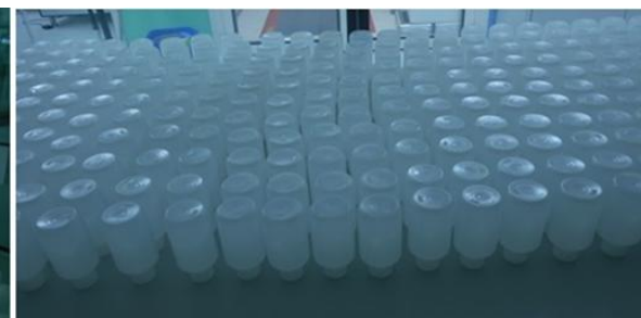
Bottle Cleaning and Drying in ISO Class 6 Clean Lab
