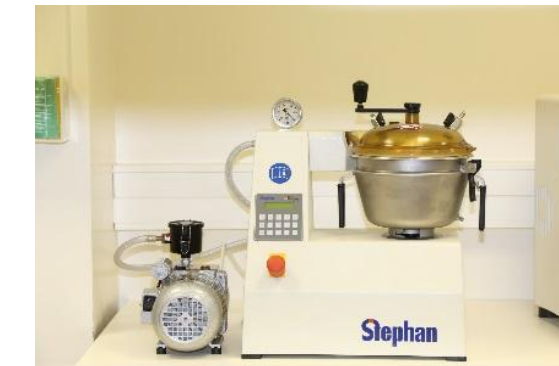
Vacuum Blender 2 Liter capacity, Stainless Steel
