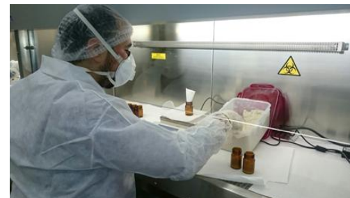
Manuel Filling Based on mass, Sticky powders Laminar Flow Cabinet
