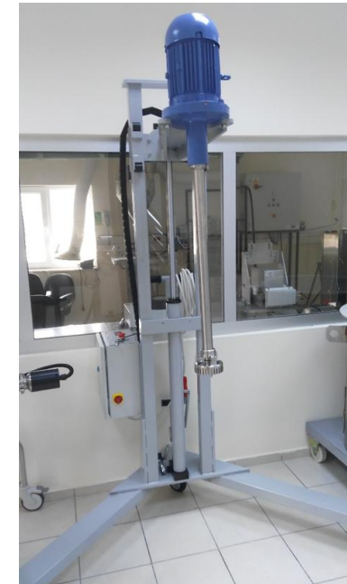
Ultraturrax Chopper Homogenizer 20-30 kg
