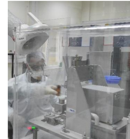
Semi Automatic Filling Based on Mass Vibration Type SS (100 mg – 10 g)
