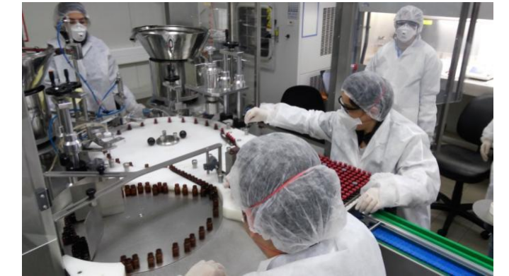
Automatic Filling Based on Peristaltic Pumping Inner capping, Screw & Crimp Capping (2 mL– 120 mL)
