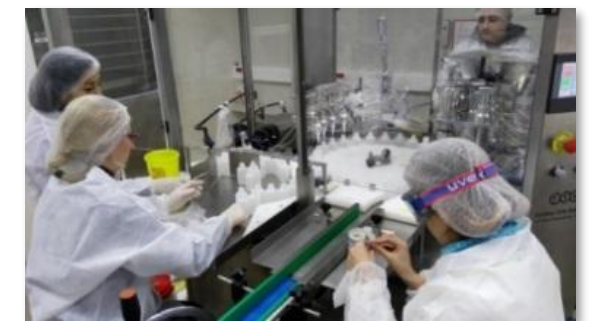
Filling and Capping
