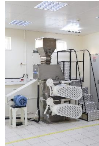
Food Grade Roller Mill 50 kg/hr, Hardened Steel
