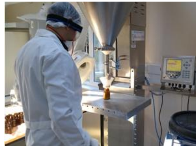
Semi Automatic Filling Based on Mass Auger Type SS/PTFE (10 g – 2 kg)
