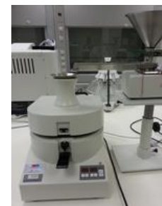
High Speed Cutting Mill 1 kg/day, Steel or Tungsten Carbide
