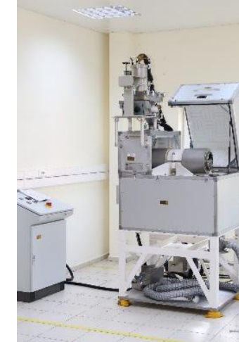
Cryogenic Titanium Mill 5 kg/day
