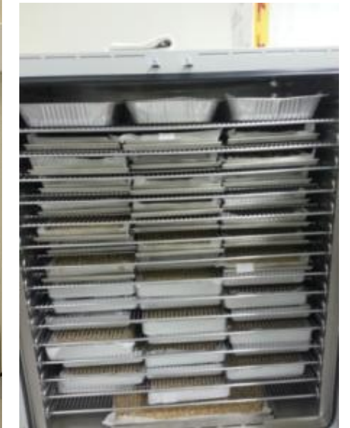
Oven with HEPA Filtered Air Flow
