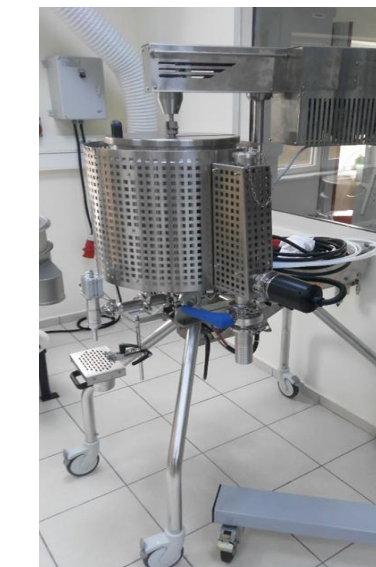
Semi Automatic Filling Based on Volume for Viscous Liquids
