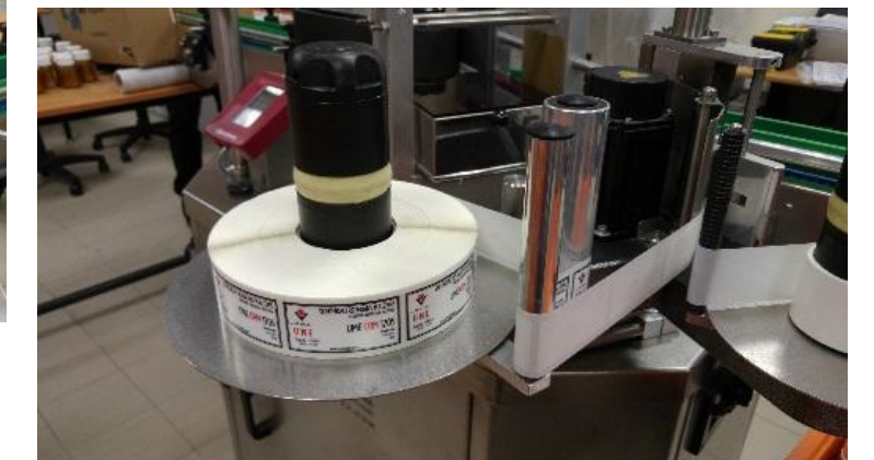
Automatic Labelling Machine For Preprinted Labels (Fill Order)
