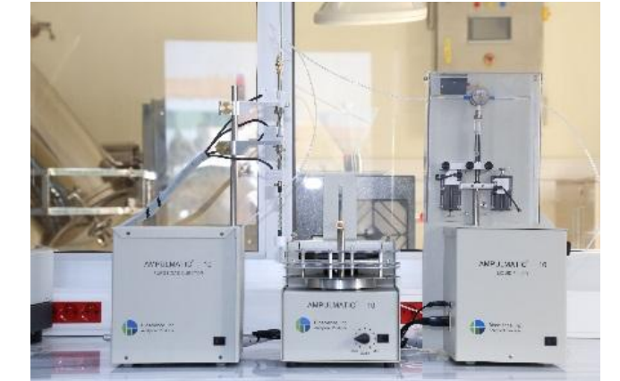
Ampouling Machine Propane-O 2 flame (1 mL– 20 mL)
