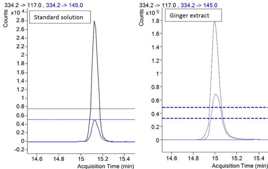
**Figure 2. Chromatograms of two transitions of tebufenpyrad in standard solution and sample. (Data from <http://www.agilent.com/cs/library/eseminars/public/Triggered%20MRM%20for%20the%20Analysis%20of%20Pesticides.pdf>)**
