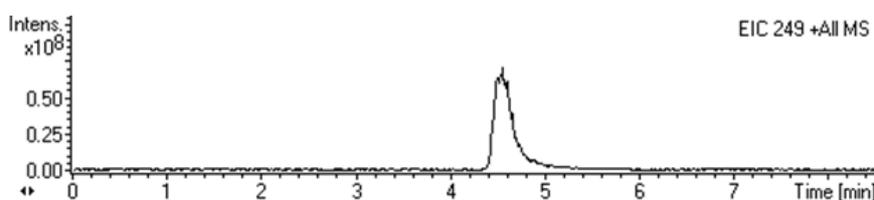
Figure 2. Extracted ion chromatogram (EIC) of Sudan I dye analysis. The  $m/z$  value 249 correspond to protonated Sudan I molecule  $[M+H]^+$ .
