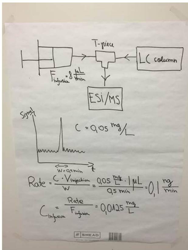
Figure 1. The experimental setup for recording the matrix effect profile.
