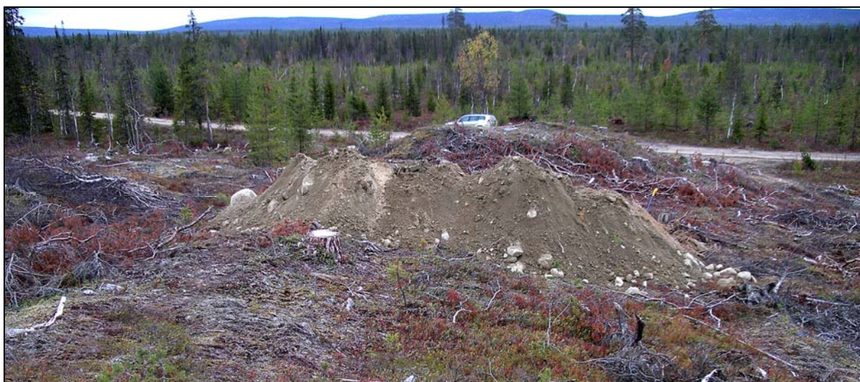
Fig. 2. A view from the end moraine ridge to the Pyhä-Luosto fell chain in the north. Sandy till material from the test pit M4 (cf. Fig. 1) is seen on a top of the ridge. Photo P. Sarala
