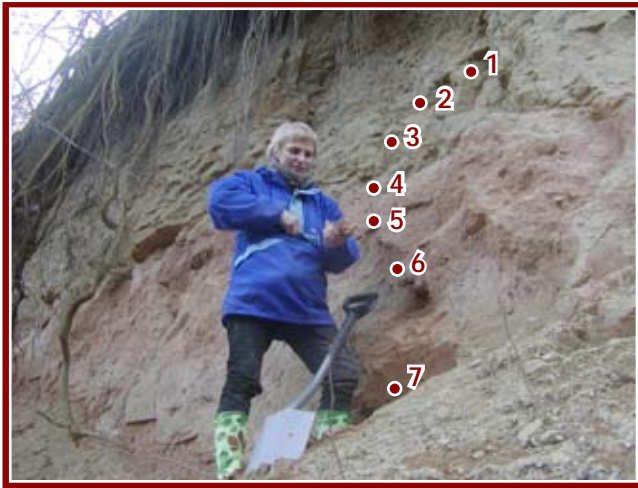
Fig. 4. The contact of brown (below) and greenish tills in the outcrop of the Karolina Ravine and sampling points for chemical and carbonate analysis presented in the Table 2
