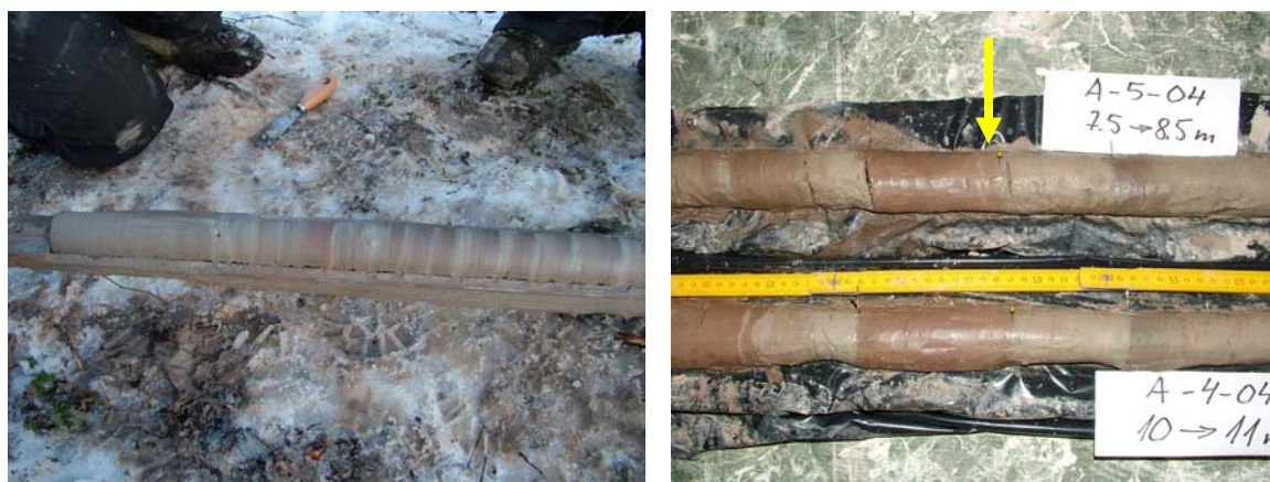
Fig 1. An example of varved clays from Pärnu area, western Estonia. Arrow points to the marker level with rapid colour change from light grey to reddish–brown on top of the series of 20 silty varves containing dispersed grains of sand. Right figure demonstrates a straight comparison of different varved sequences for varve correlation.
