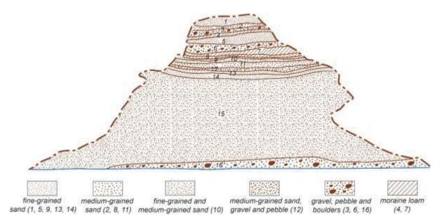
Fig. 4. Sediment layers recorded by ground-based geodetic measurements.
