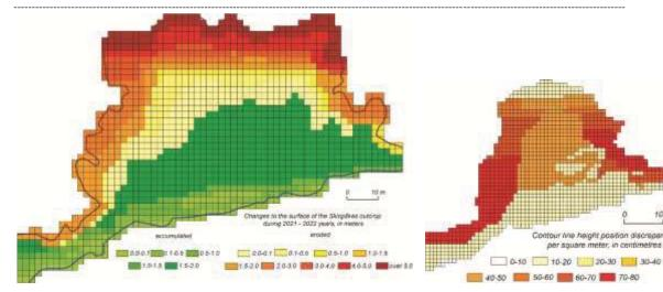
**Fig. 2.** Erosion and accumulation zones on the Skirgiškės outcrop 2021 – 2022 years (choropleth method).
