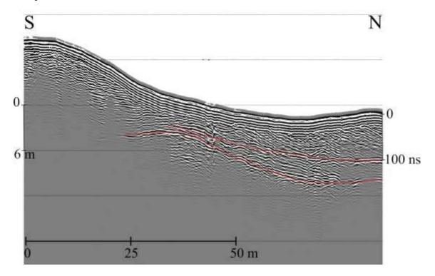
Fig. 2. Ground-penetrating radar profile close to the railway bridge near Zervynos village.
