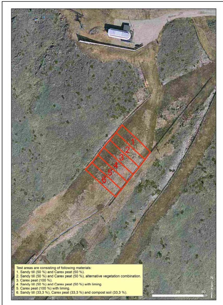
Fig. 5. Test areas near top of the Levi, locating on a block field.
