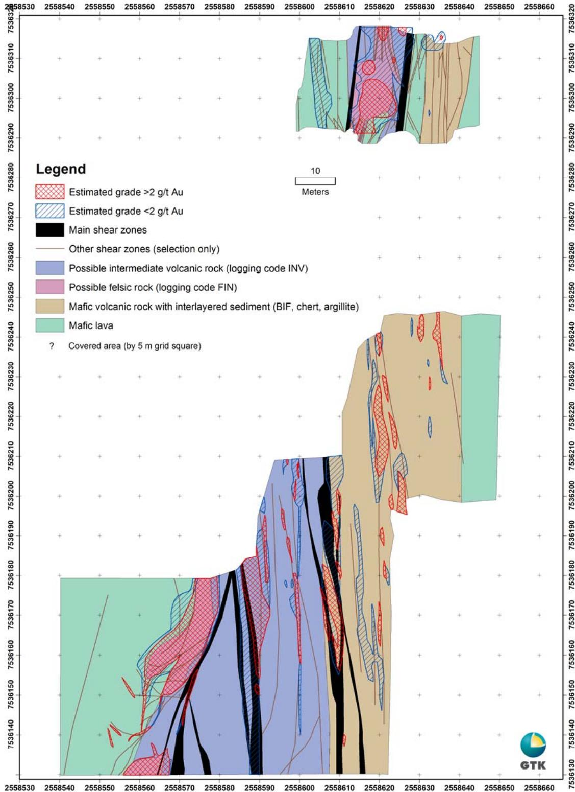
Fig. 14. Pit map from Suurikuusikko showing the main rock types and structures, in 10 m grid (after Patison *et al.* 2006). The grade estimates shown are visual estimates based on arsenopyrite abundance. Exposure of the deposit prior to 2007 was limited to the two pits shown in this figure.
