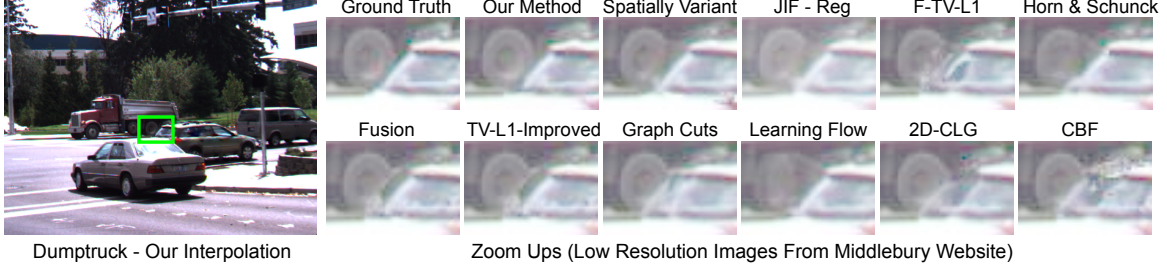
Figure 7: Comparison with optical flow algorithms from Middlebury website on Dumptruck dataset. We show the brightness enhanced zoom-ups of the marked region along with the ground truth and top ten optical flow methods from the website on these images. We are able to handle occlusions well and preserve the frequency content. Note the blurring of tires and the ghosting on the back window visible in other methods.
