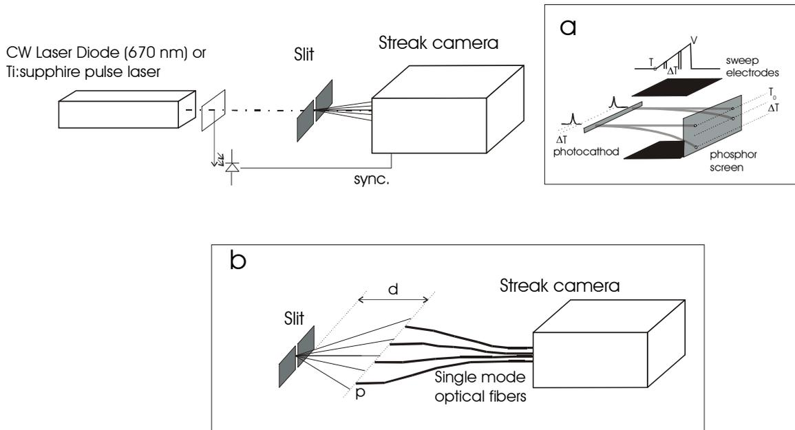
**Figure 1** Experimental arrangement. A sketch of the way the diffraction experiments are performed. A CW diode-laser (670nm) or Ti:sapphire femtosecond pulsed laser was used as a source of light.
