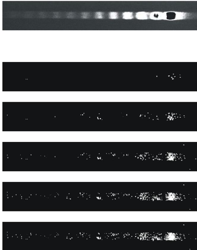
**Figure 2** Diffraction pattern taken from a slit ( $150\ \mu\text{m}$  width) with zero-order maximum left out (because of extremely high intensity, i.e. saturation). No sweep voltage was applied to the streak camera electrodes, so the frames are just images of the streak camera input window. Top frame was taken in analogue mode. Others frames were taken in photon counting mode and correspond to 10, 50, 120, 240, 300 photoelectrons.
