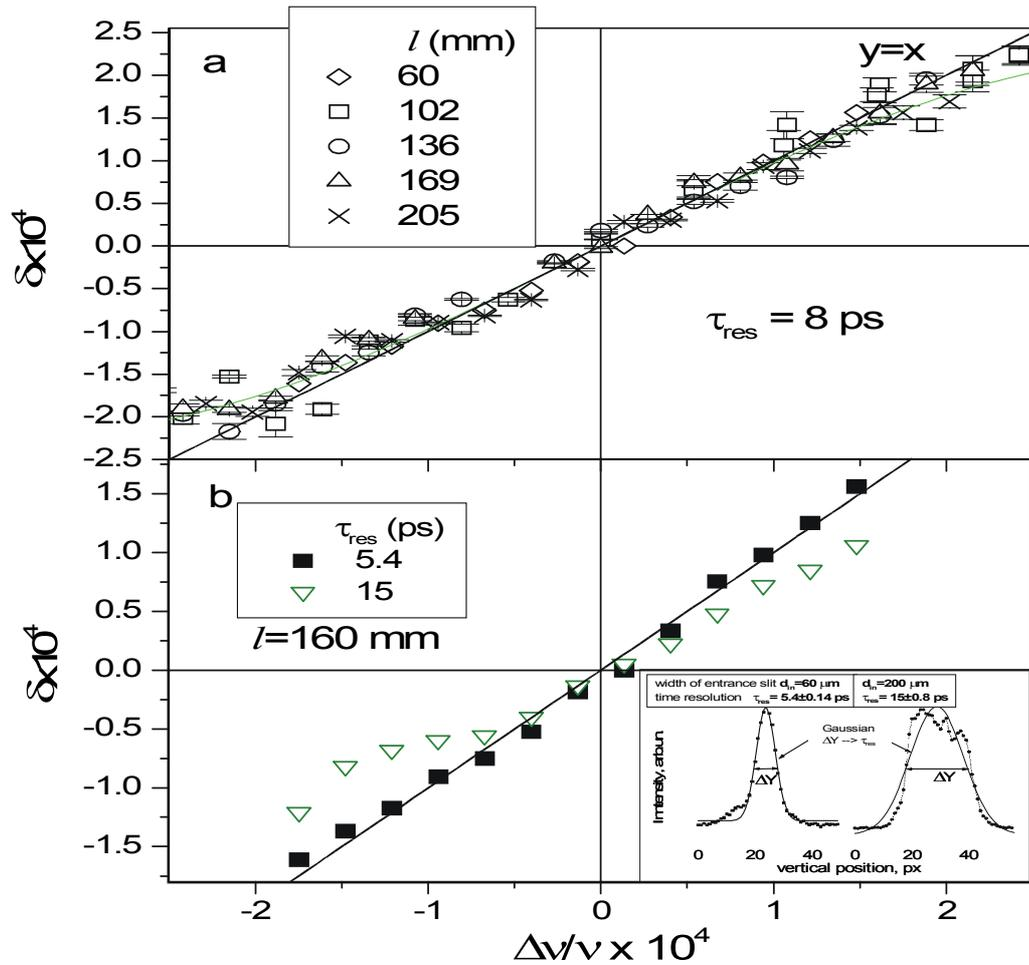
**Figure 6** Dependence of the normalized slope of the interference fringes on the relative difference of frequency of light in the fibres. Points are experimental data, lines are calculated using classical theory for addition of two waves Eq.(3).
