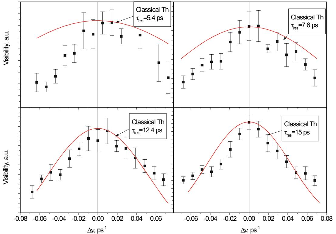
**Figure 8** Visibility of interference fringes vs. frequency differences of light beams. Experimental data (points), and calculated curves correspond to different time resolution values  $\tau_{res}$  of the streak camera.
