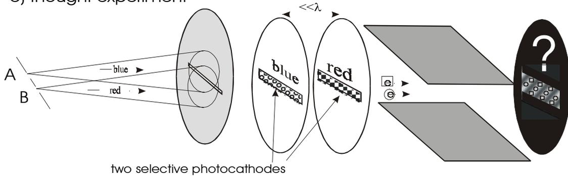
Figure A a) Sketch of the streak camera arrangement; b) arrangement for the interference experiments shown in this work. The cathode cannot distinguish the colour being insensitive to small frequency differences. In this case we see fringes. c) The new photocathode design for a thought experiment. We have two photocathode plates separated by a distance much smaller than  $\lambda$  in such a way that the pulses overlap but now one plate signs blue and the other red.
