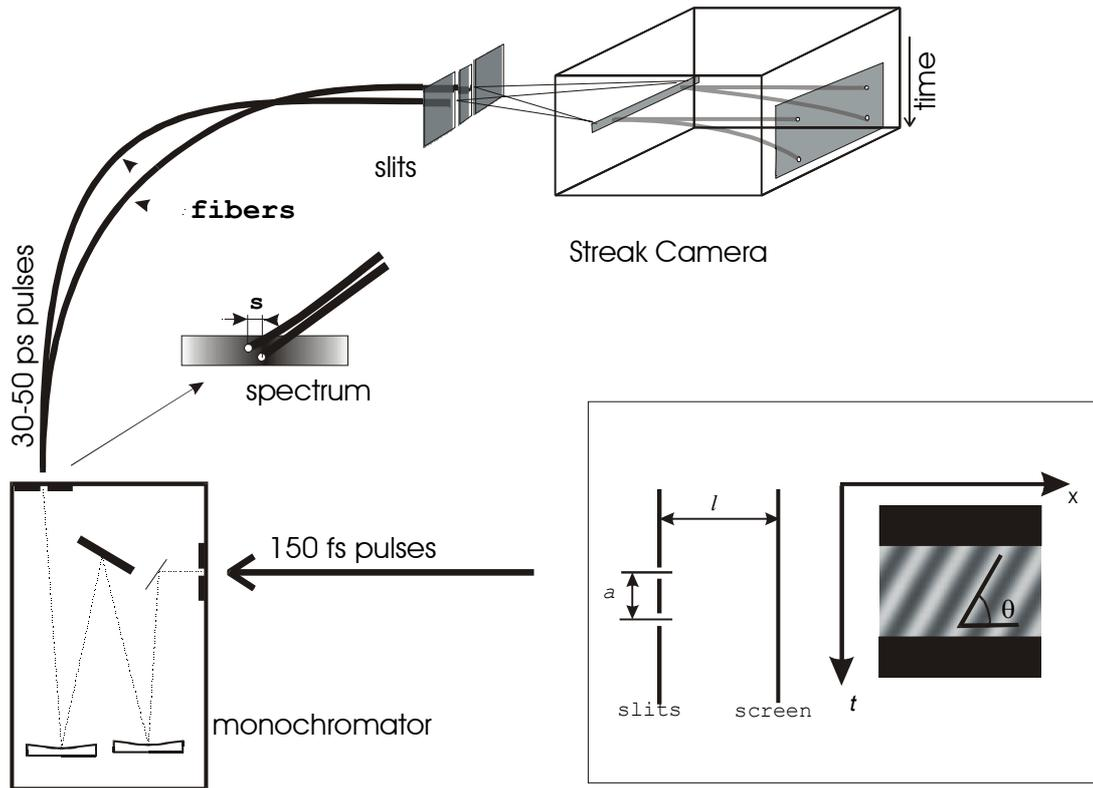
**Figure 4** Arrangement for the interference experiments.
